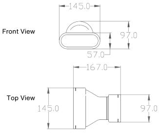
Zehnder ComfoTube Flat 51 to Zehnder ComfoTube ø 90 mm, 90° convertor
