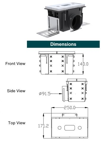
Grille housing TVA-P 90 connects 1 x ø 125 mm valve to 2 x ø 90 mm Zehnder ComfoTube, L300 mm
