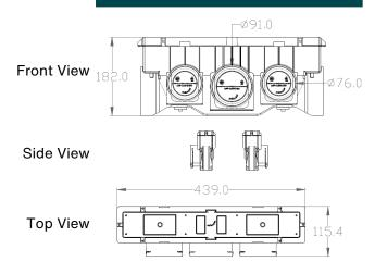
Rectangular grille housing CSB-P 600 connects 1 x Lamina/Bilamina/ComfoGrid 600 to 1 x ø 110 mm, 2 x ø 90 mm Zehnder ComfoTube
