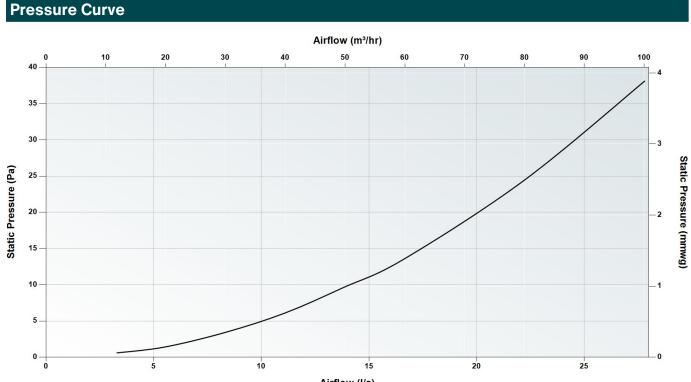
Airflow (I/s) ----- Zehnder ComfoFresh Flat 51 to Zehnder ComfoTube ø 90 mm, 90° convertor
