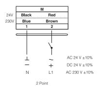
↑ Connect via safety isolating transformer
